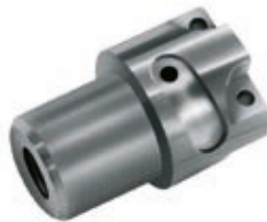
Part with 4axis milling operations
