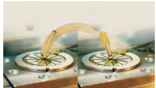
Part turn-over in different section collet
